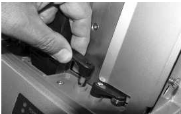
Picture 6.5 Adjust the pressure of turning arm
