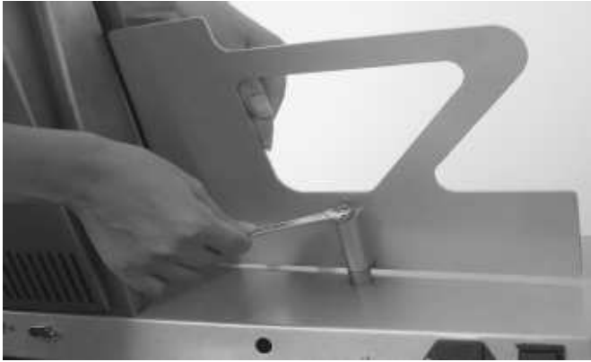
Picture 6.7 Input stacker and fixing screw
