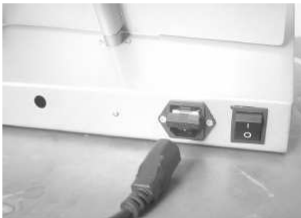
Picture 6.2 Power socket and insurance pipe
