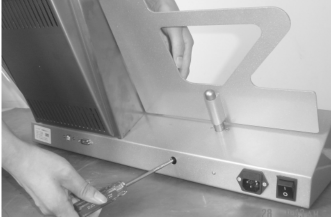
Picture 6.6 Adjust the thrust of the bracing board
